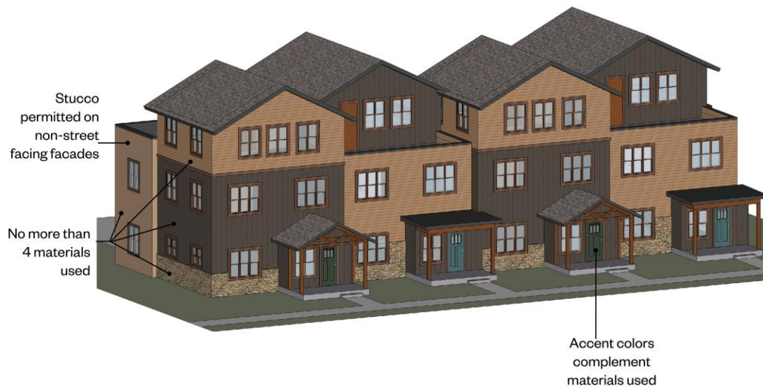
Multi-Family Building Materials with Alley Access Diagram.
