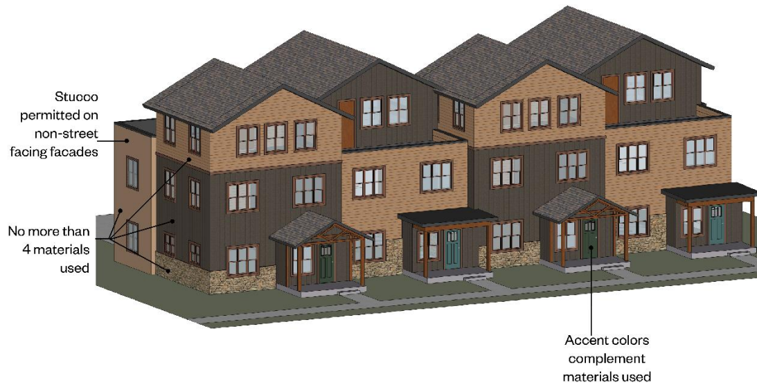
Multi-Family Building Materials with Alley Access Diagram.
