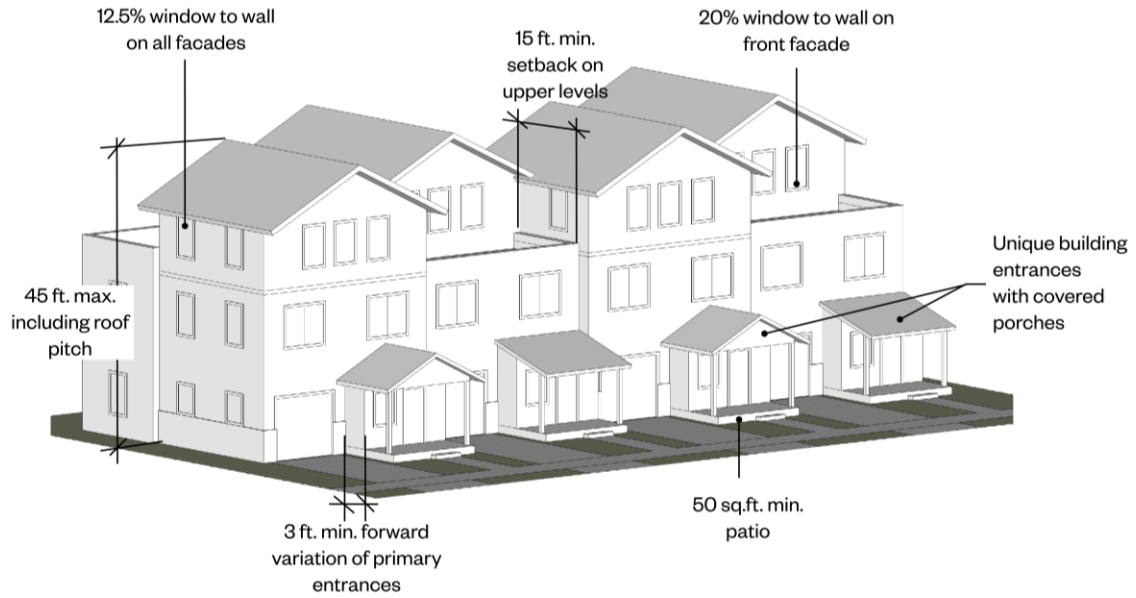
Multi-Family Building Height, Massing, Articulation, and Architectural Detail with Front Garages Diagram.
