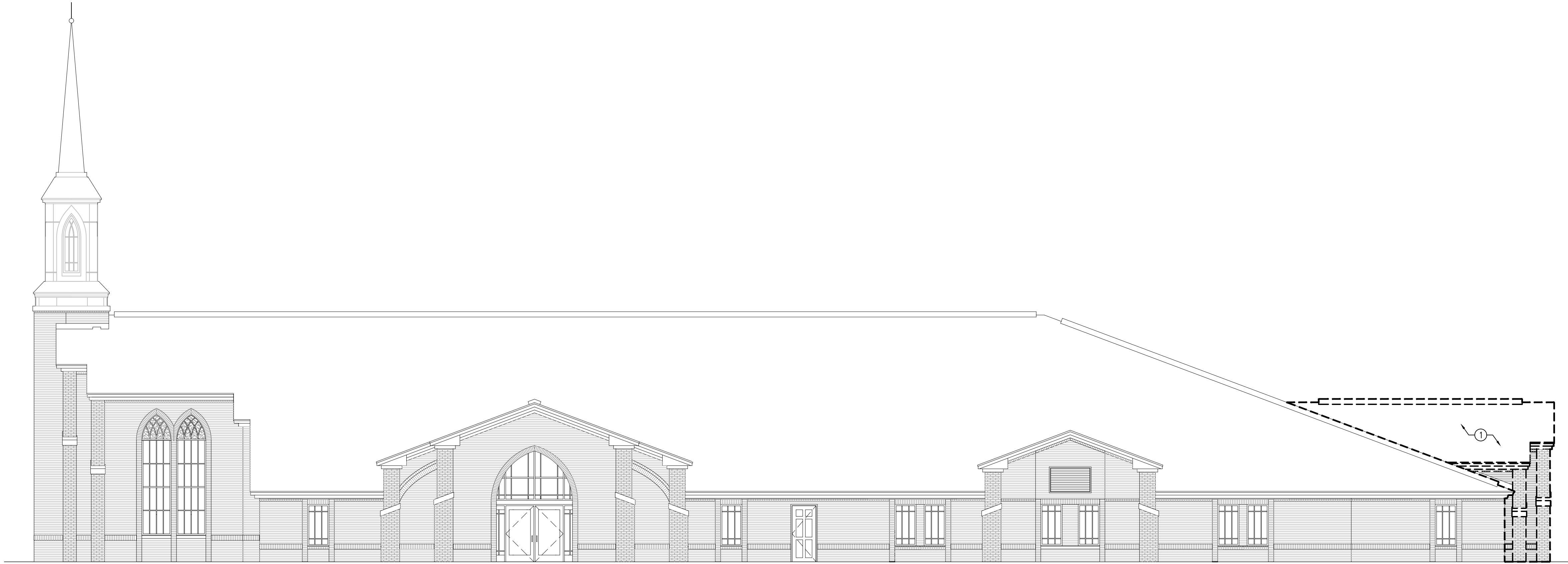
A DEMOLITION SOUTH ELEVATION SCALE: 1/8" = 1'-0"
