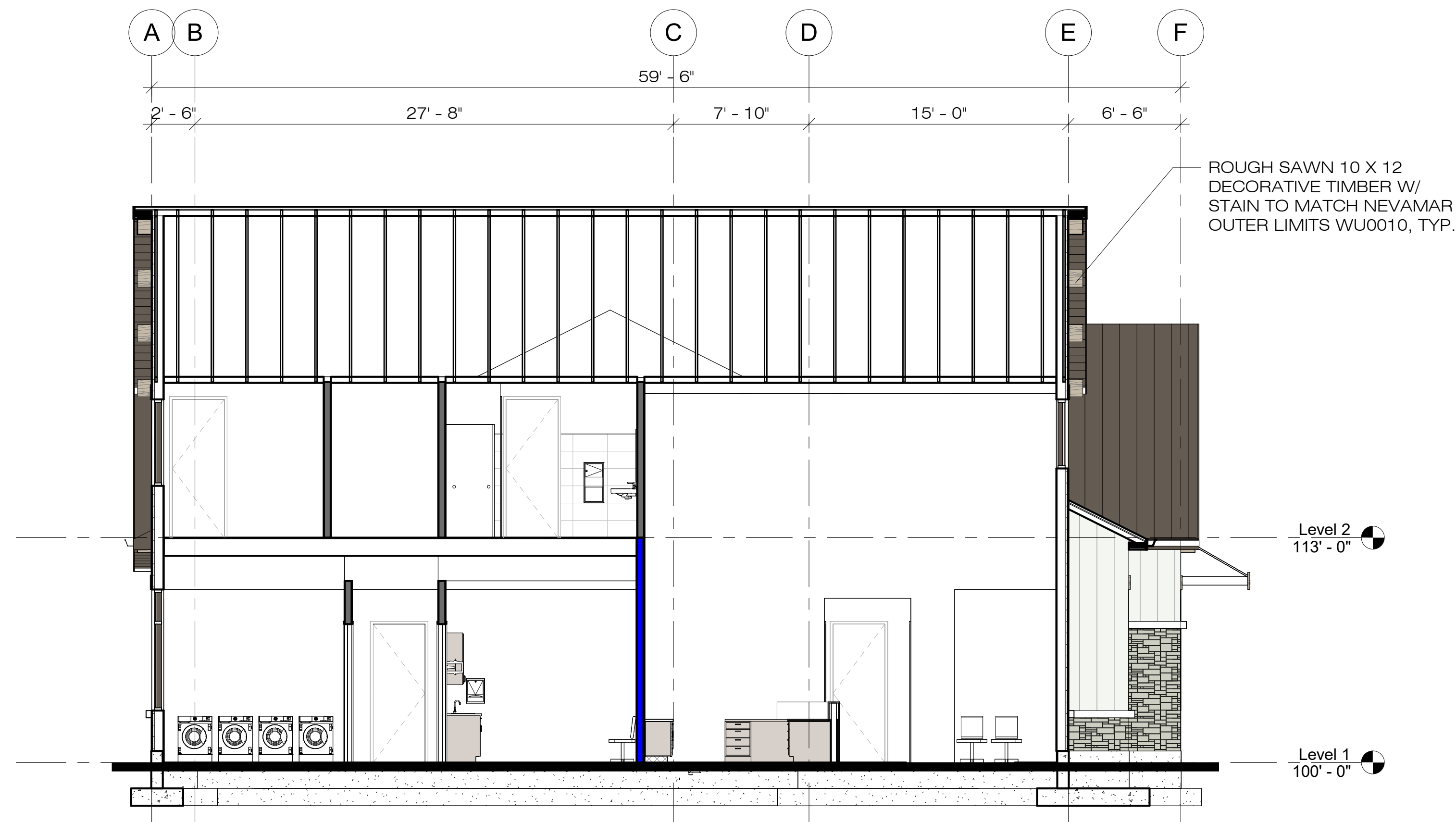
2 BUILDING SECTION SCALE: 3/16" = 1'-0"
