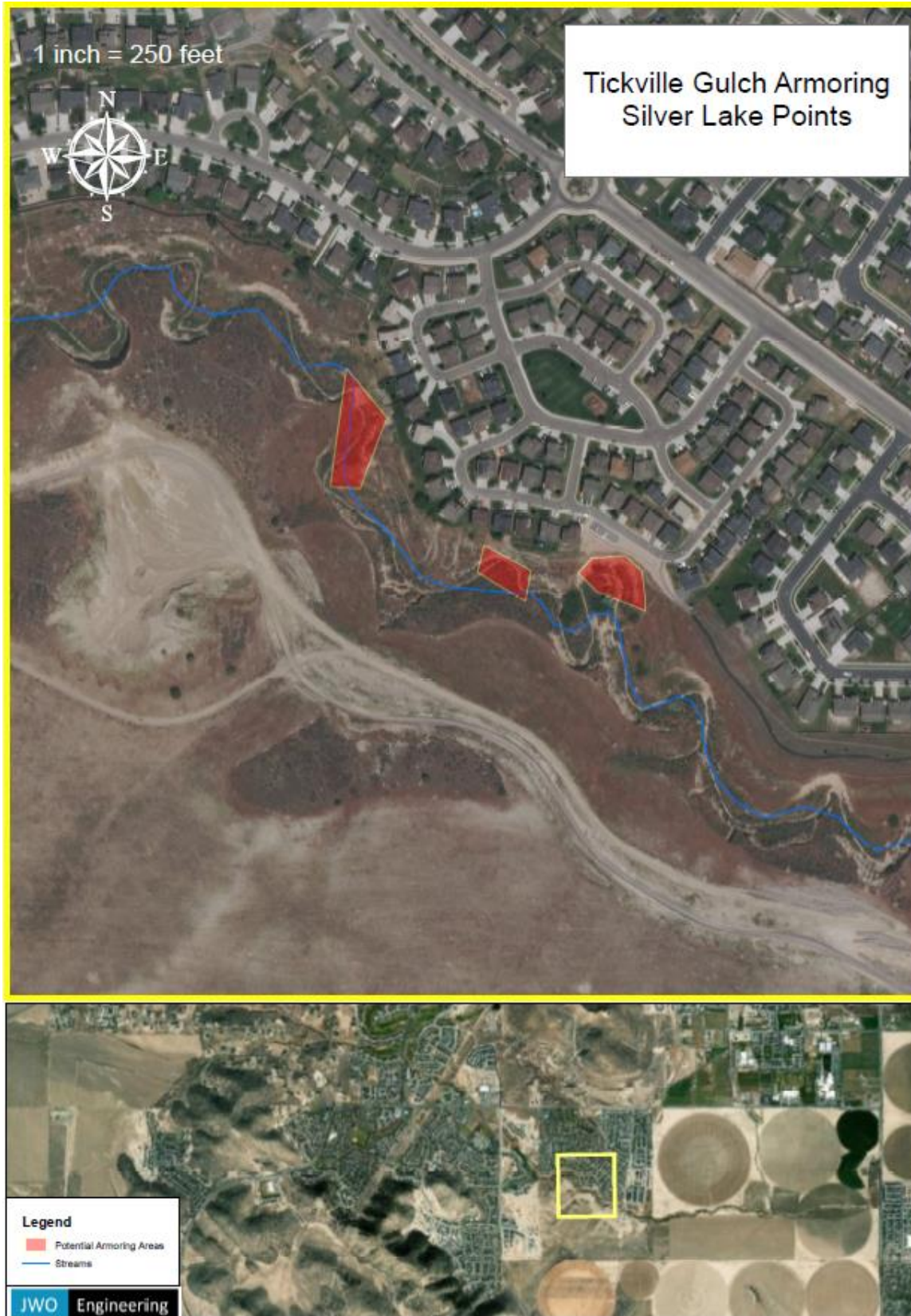
Figure 7. Potential armoring areas along Tickville Wash near Silver Lake Subdivision
