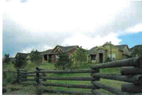
Open rail fencing may have pet mesh (hogwire) attached to the inside, but should otherwise remain visually open
